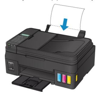
After loading paper on the rear tray, the paper information registration screen appears on the LCD. Select **A4** or **Letter** for **Size:** and **Plain paper** for **Type:** and then press the **OK** button.
