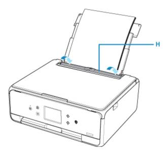
After closing the feed slot cover, the paper information registration screen for the rear tray is displayed on the touch screen.
