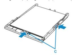
5. Mount the cassette cover, and then insert the cassette into the printer.
