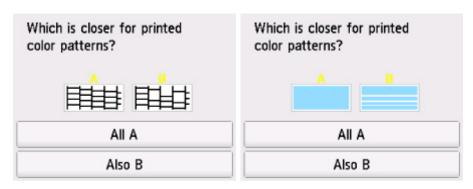
For A (no missing lines or no horizontal white streaks) in both the pattern C and pattern D:
