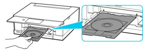
**4.** Insert multi-purpose tray straight in in horizontal direction until arrow (**∑**) on multi-purpose tray guide is approximately aligned with arrow (**∑**) on multi-purpose tray.
