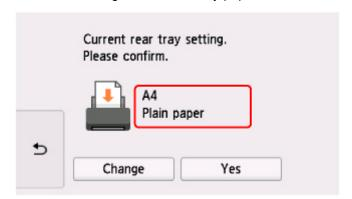
If the page size on the touch screen matches the size of the paper loaded in the rear tray, select **Yes**. If not, select **Change** to change the setting in accordance with the size of the loaded paper.
