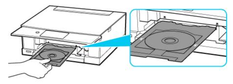
**15.** Insert multi-purpose tray straight in in horizontal direction until arrow ( $\stackrel{\checkmark}{}$ ) on multi-purpose tray guide is approximately aligned with arrow ( $\stackrel{\checkmark}{}$ ) on multi-purpose tray.
