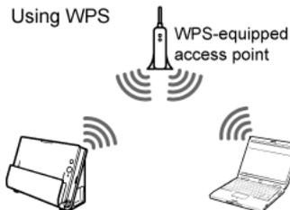
If the wireless access point is WPS-compatible, connection to the scanner can be made using the WPS feature.
