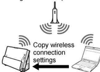
Connection to the scanner can be made using the wireless settings of the computer connected to the wireless LAN access point.
