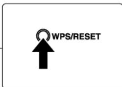
This scanner begins communicating with the connection-waiting access point to automatically configure the required Wi-Fi settings. When the settings are configured, the CONNECTION lamp lights steadily (green).
