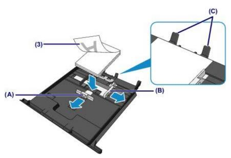
(4) Align the paper guide (A) in front with the paper stack. For standard sizes, align the paper guide (A) with where it clicks into place.
