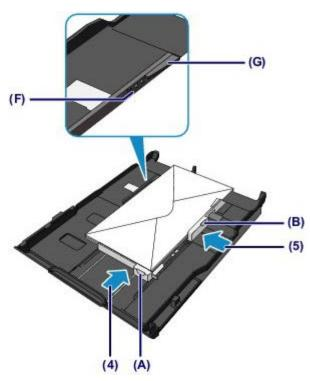
(6) Insert the cassette (lower) into the printer. Push the cassette (lower) into the printer until it stops.
