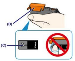
(3) Lift up the tab on the orange protective cap (D) to remove it off GENTLY.
