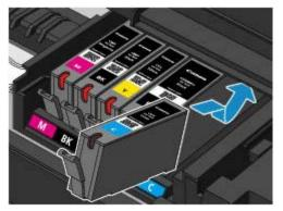
(2) Press on the top of the ink tank until the ink tank snaps firmly into place. Make sure that the ink lamp lights up red.
