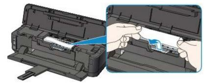
**5.** Pull the paper slowly not to tear it, then pull the paper out diagonally forward in front at aslant.
