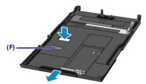
The cassette (lower) sticks out of the printer when correctly set. Do not force the cassette (lower) into the printer any further.
