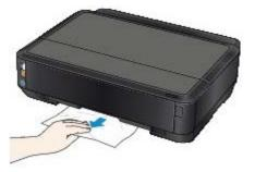
**8.** If the paper is not loaded properly in the cassette, remove the paper, then reload it after aligning the edges of the sheets.
