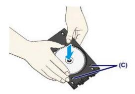
**5.** Attach the disc tray to the printer.
