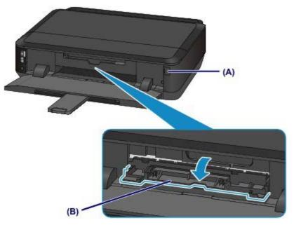
4. Place the printable disc with the printable surface facing up.
