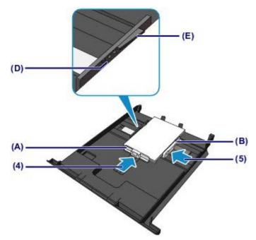
(6) Insert the cassette (upper) into the printer. Push the cassette (upper) all the way into the printer.
