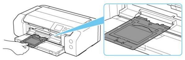
6. Insert multi-purpose tray straight in in horizontal direction until arrow (∑) on multi-purpose tray guide is approximately aligned with arrow (乙) on multi-purpose tray.
