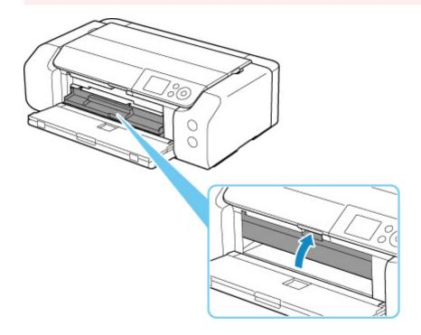
**3.** While pressing down lock (A), take out printable disc from slits (B) on multi-purpose tray, and remove it.
