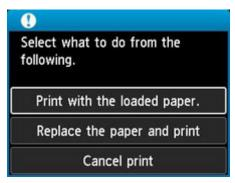
Select the appropriate action using the  $\blacktriangle \nabla$  buttons and press the printer's **OK** button.
