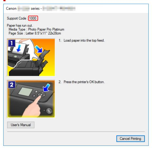
When a Support Code and a Message are displayed on the Printer's LCD:
