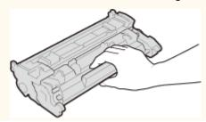
• Do not touch the toner cartridge memory (a) or the electrical contacts (b). To avoid scratching the surface of the drum inside the machine or exposing it to light, do not open the drum protective shutter (c).
