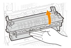
**2** Pull out the lever with the green mark on the left side of the delivery guide.
