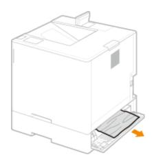
**6** Pull out the paper drawer of the paper feeder, and gently pull out the paper.
