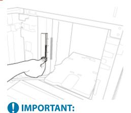
• Make sure to align the lever with the mark for the size of the paper to load. Setting the lever in a different position may result in a paper jam.
