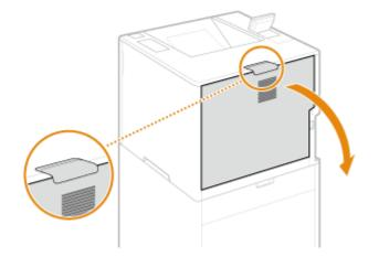
**2** Remove the jammed paper in the delivery unit.
