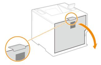
**2** Remove the jammed paper in the delivery unit.
