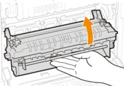
Pull out the lever with the green mark on the left side of the delivery guide.
