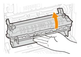
2 Pull out the lever with the green mark on the left side of the delivery guide.
