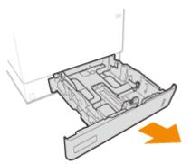
When loading LGL size paper, pull out the front panel.
