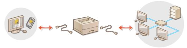
1 Connect the USB-LAN adapter to the USB port of the machine (front-right side of the machine). **Parts** and Their Functions(P. 52)
