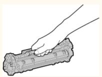
Do not scratch the drum surface (a) or expose it to light. Also, do not touch the electrical contacts (b) or the toner cartridge memory ( ).
