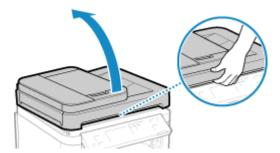
Place the side of the original to be scanned face down on the platen glass in the landscape orientation while aligning the corner of the original with the top left corner of the platen glass.
