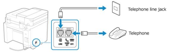
Connect the telephone to the external telephone jack (EXT.) on the machine.
