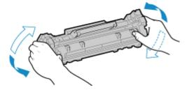
6 Remove the protective cover of the toner cartridge.
