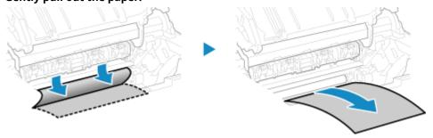
Holding both sides of the paper, pull the front edge of the paper out and downwards.
