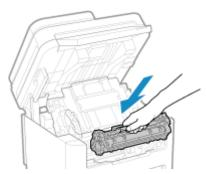
The bottom of the toner cartridge is unprotected. Be careful not to bump the bottom of the toner cartridge against the slot frame or other parts when installing.
