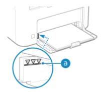
• Check that the paper guides are aligned with the markings and are not too loose or too tight.
