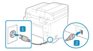
3 Unplug all cables and cords connected to the machine.
