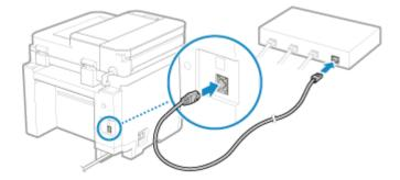
Insert the connector all the way into the port until it clicks in place.
