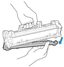
Be careful not to touch the drum surface on the bottom of the toner cartridge.
