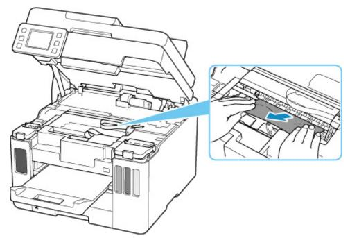
If the paper is rolled up, pull it out and grasp the edges of the paper.
