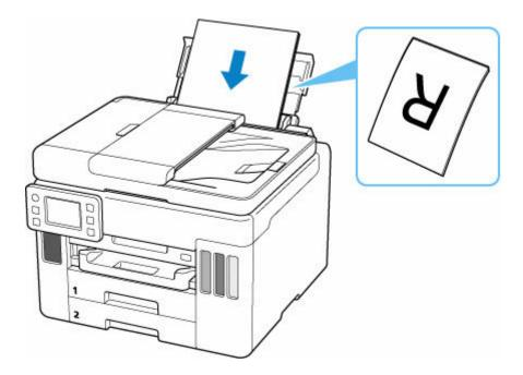
**5.** Slide right paper guide to align with both sides of paper stack.
