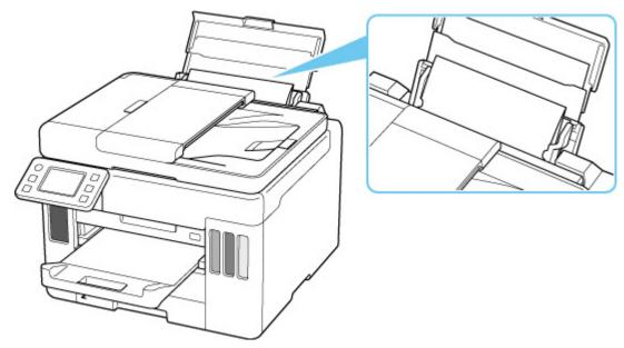
3. Remove foreign object by hand with paper inserted.
