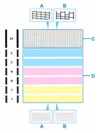
A: No missing lines/No horizontal streaks
