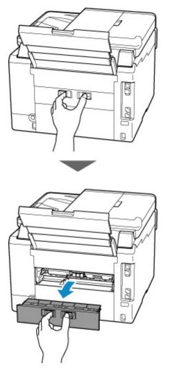
**6.** Hold jammed paper firmly with both hands and pull it out slowly. If the paper is rolled up, pull it out and grasp the edges of the paper.
