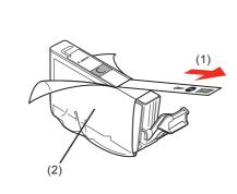
Pull the orange tape (1) in the direction of the arrow to peel off the protective film and remove the film (2) completely.
