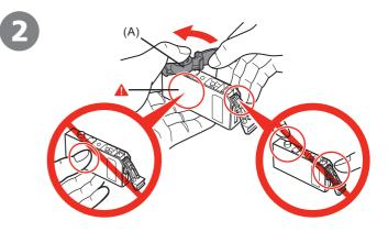
While pressing down with your left thumb, twist off the orange protective cap (A) located on the bottom of the ink tank.
