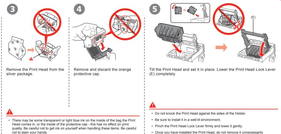
· Once you have installed the Print Head, do not remove it unnecessarily.
