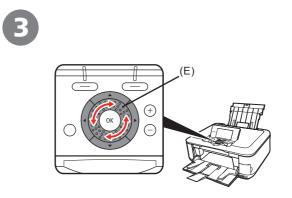
Rotate the Easy-Scroll Wheel (E) to display a photo to print.
