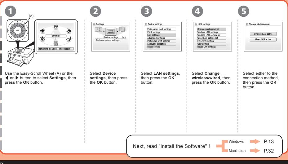
Setup the Machine and the Computer
