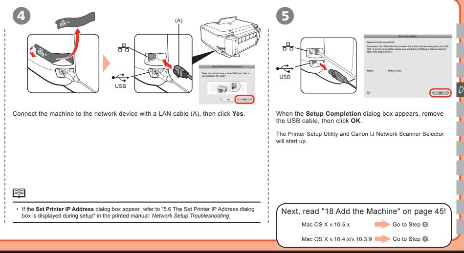
Setup the Machine and the Computer
