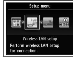
Use the ◀ or ▶ button (C) to select **Wireless LAN setup**, then touch the **OK** button.
