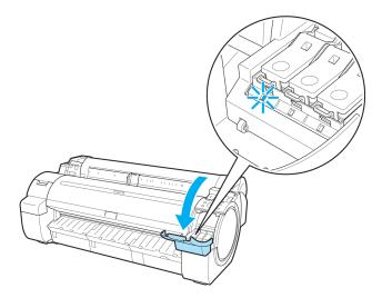
Press the tip of the Ink Tank Lock Lever of the color for replacement horizontally and pull the Ink Tank Lock Lever up to open it.
