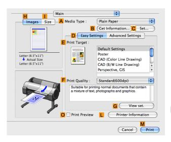
In the Paper Detailed Settings dialog box displayed next, select the desired settings values in C Between Pages and D Between Scans in B Drying Time, and then click OK.
