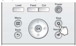
When you press the **Stop** button during printing, printer operation varies depending on the current status.
