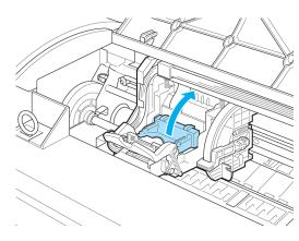
5 Remove the Printhead and press the **OK** button.
