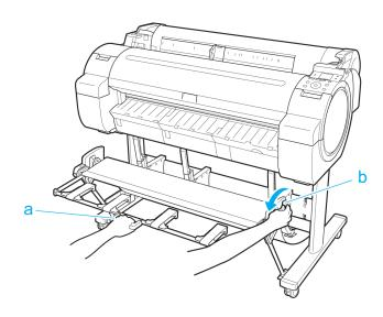
While continuing to hold the Output stacker handle (a), slowly lower the Output Stacker.
