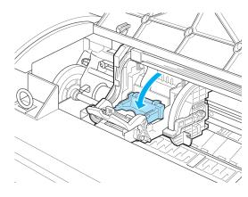
10 Push the Printhead Fixer Lever toward the back of the printer until it clicks.
