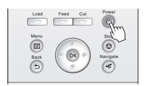
The **Power Lamp** is lit when the printer finishes starting up, and the printer is now in **Standby**.
