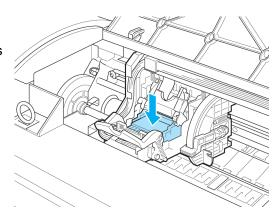
9 Pull the Printhead Fixer Cover down toward the front to lock the Printhead in place.
