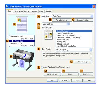
In the A Media Type list, select the type of paper that is loaded. In this case, click Premium Glossy Paper 200. In the A Media Type, choose the type of paper used for printing, such as Glossy Paper, Coated Paper, and so on. Make sure the paper you select is loaded in the printer.
