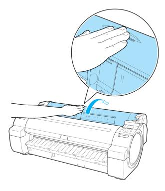
Using both hands, rotate the Roll Holder toward the back to rewind the roll.
