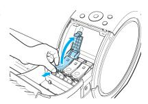
3 Hold the lnk Tank by the grips and remove it. Press the **OK** button.
