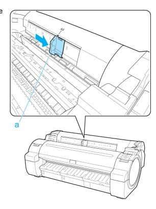
3 Load a single sheet printing-side up in the Paper Feed Slot, with the right edge aligned with the Paper Alignment Guide (a) to the right of the Roll Cover. Insert the paper until the leading edge makes contact and you hear a tone.
