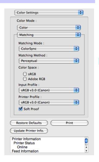
2 Place a checkmark on **Soft Proof** to simulate the output product in Layout Area.
