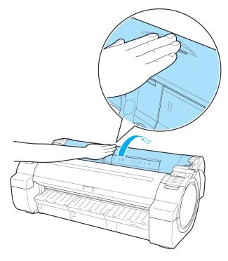
Fold an A4 sheet lengthwise four times and insert it through the gap of the Paper Feed Slot. Push the scrap out toward the Platen.
