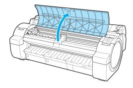
7 Align the Angle Adjustment Lever with the red square and close the Top Cover.
