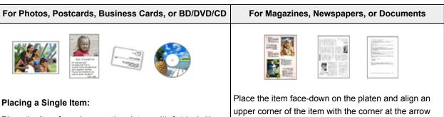
Place the item face-down on the platen, with 0.4 inch (1 cm) or more space between the edges (diagonally striped area) of the platen and the item. Portions placed on the diagonally striped area cannot be scanned.
