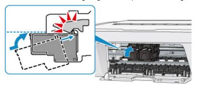
After confirming that the FINE cartridge is installed properly, close the cover.
