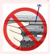
If the paper or your hands touch the clear film and blot or scratch it, the machine can be damaged.
