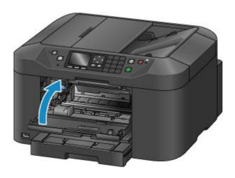
After replacing the ink tanks, the machine starts mixing the ink automatically. Wait until the machine has stopped making operating noise. (This takes about 1 to 2 minutes.)
