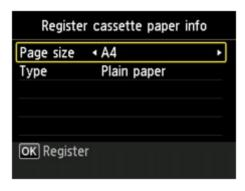
Press the machine's **OK** button to terminate the paper settings of the cassette.
