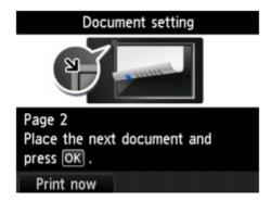
Remove the first sheet of original from the platen glass and load the second sheet on the platen glass, then press the **OK** button.
