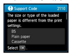
Confirm the message, then press the **OK** button. When the screen to select the operation is displayed, select one of the operations below.
