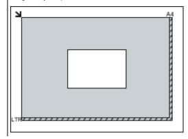
Place the item face-down on the platen and align an upper corner of the item with the corner at the arrow (alignment mark) of the platen. Portions placed on the diagonally striped area cannot be scanned.
