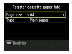
Register the paper size and the media type according to the loaded paper.
