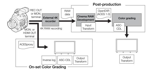
ACESproxy video data that is output from the MON. terminal or HDMI OUT terminal when
