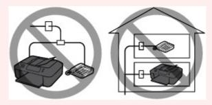
If you cannot avoid parallel connections, set the receive mode to **TEL priority mode**, understanding that the above problems may occur. You will only be able to receive faxes manually.
