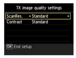
2. Use the ▲▼ button to change the setting item and use the ◀▶ button to change the setting. The following settings are selectable on **ScanRes.**.
