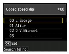
3. Use the **ATIN** button or the Numeric buttons to select a coded speed dial code to register to the group dial.
