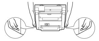
Pull out the cassette completely, and remove the extension cover. Detach the output tray.
