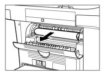
7 Carefully pull the jammed paper straight out through the rollers.
