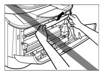
6 Gently pull the jammed paper between the output rollers until the leading edge emerges from the machine.
