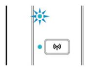
If the **Wireless** lamp is not lit, the printer is not connected to the wireless router. Check the environment or settings of the wireless router.
