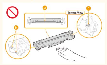
• Except when necessary, do not take out the drum cartridge from the packing material or from this machine.
