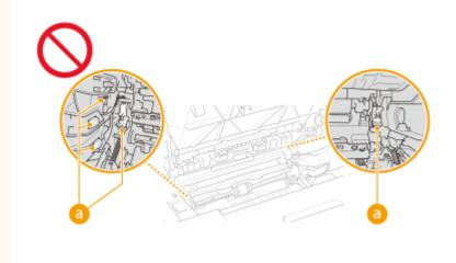
• To prevent a paper jam, do not turn OFF the power, open/close the covers, and load/unload the paper when printing.
