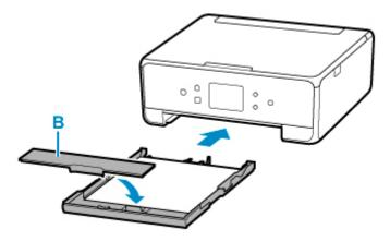
After inserting the cassette into the printer, the paper setting confirmation screen for the cassette appears on the touch screen.
