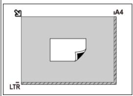
upper corner of the item with the corner at the arrow (alignment mark) of the platen. Portions placed on the diagonally striped area cannot be scanned.
