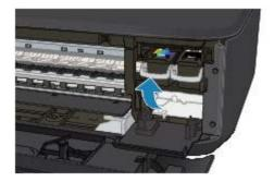
After confirming that the FINE cartridge is installed properly, close the paper output cover. If the problem is not resolved, remove the FINE cartridges, then install them again.
