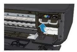
After confirming that the FINE cartridge is installed properly, close the paper output cover.
