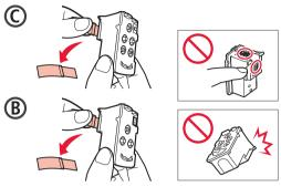
4 Insert the C (color) print head on the left and the B (black) print head on the right.
