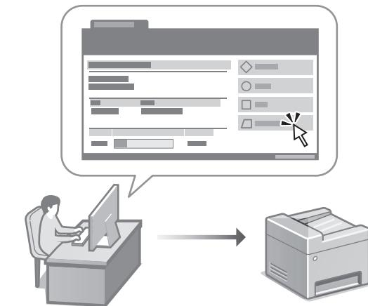
Remote UI allows this machine to be managed using the Web browser on a computer. You can use it to check the machine's operating status, change settings, and save items to the Address Book.
