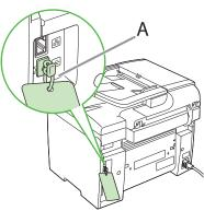
The machine has a cap (A) that covers the USB port on the back of the machine. Remove the cap (A) by pulling the string.
