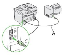
After restarting your computer, connect the machine and your computer with a USB cable (A).
