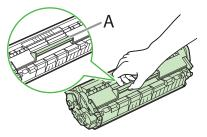
**9** Insert the toner cartridge so that the protrusion on the right side of the toner cartridge (A) fits into the guide (B) located on the right side of the machine and slide it down parallel to the guide.
