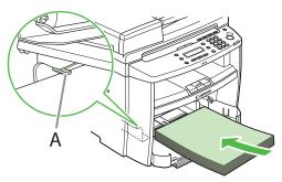
8 Adjust the paper guide rail to match the size of paper.
