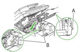
**10** Push the toner cartridge to make sure it is properly set in the machine.
