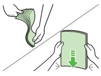
7 Load the paper into the paper cassette with the print side up. Make sure the paper stack sits below the small fin (A) on the side paper guide.
