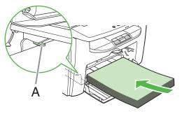
**7** Adjust the paper guide rail to match the size of paper.
