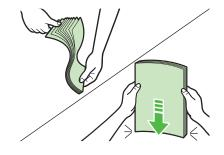
**6** Load the paper into the paper feeding tray with the print side up. Make sure the paper stack sits below the hook (A) on the side paper guide.
