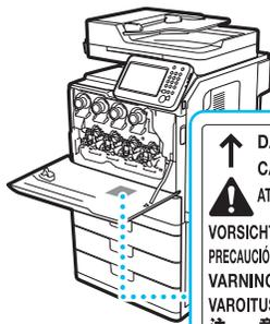
↑ **DANGER** - Invisible laser radiation when open and interlocks defeated. AVOID DIRECT EXPOSURE TO BEAM.
