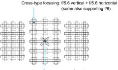
Dual cross-type focusing: f/2.8 right diagonal + f/2.8 left diagonal f/5.6 vertical + f/5.6 horizontal (also supporting f/8)
