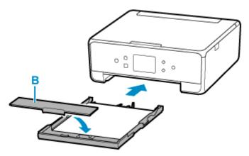
After inserting the cassette into the printer, the paper setting confirmation screen for the cassette appears on the touch screen.
