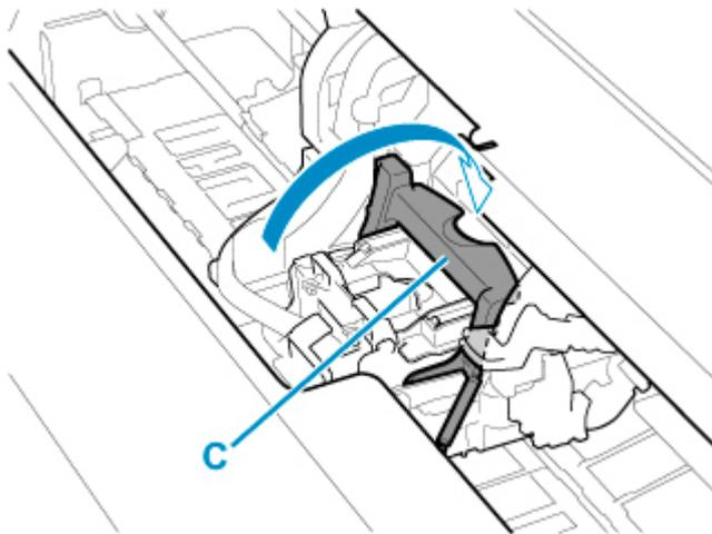
**14.** Align angle adjustment lever with the red square position.
