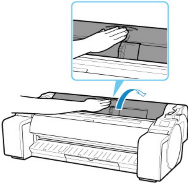
**3.** Using both hands, rotate the roll holder toward the back to rewind the roll.
