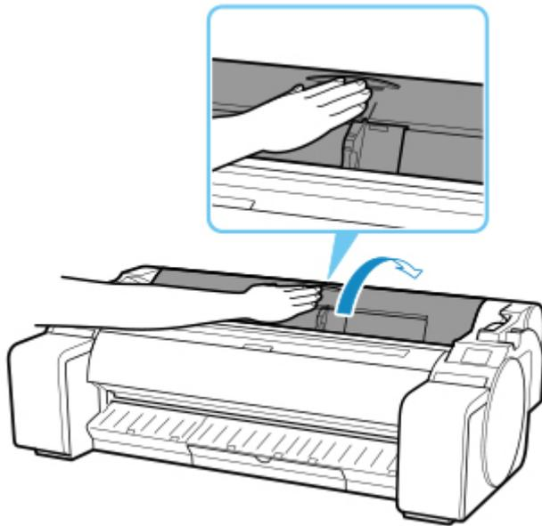
5. Using both hands, rotate the roll holder toward the back to rewind the roll.
