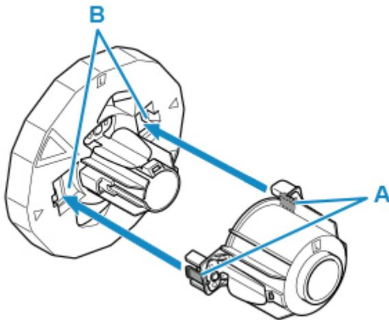
5. Insert holder stopper from left into roll holder as shown, and then while holding in position (B), push firmly until holder stopper flange (A) touches roll paper. Lock the holder stopper lever (C) by rotating it towards
