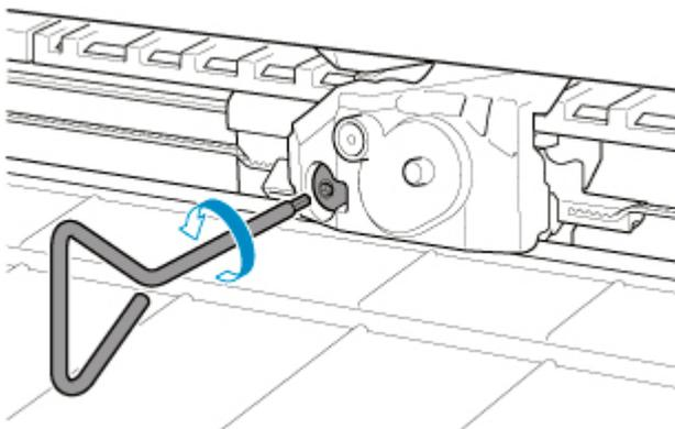
6. Remove cutter blade while holding A.
