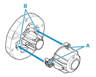
5. Insert holder stopper from left into roll holder as shown, and then while holding in position (B), push firmly until holder stopper flange (A) touches roll paper. Lock the holder stopper lever (C) by rotating it towards .
