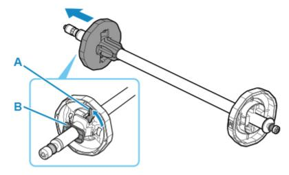
**2.** If using 3-inch core paper, align 3-inch paper core attachment R tabs (A) with roll holder holes (B) and insert firmly.
