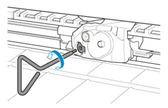
6. Remove cutter blade while holding A.
