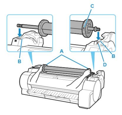
**4.** Holding the roll holder flange (A), guide the holder along the slide guides (B) on both ends, keeping the holder level as you load it in the roll holder slot.
