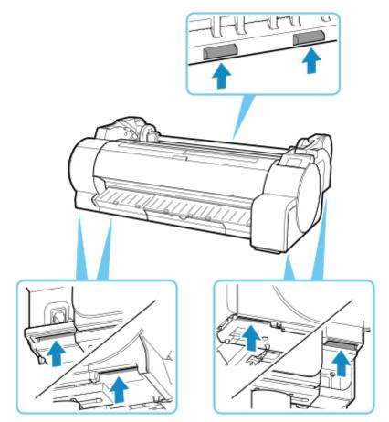
• When placing the printer on the stand, lock all four of the casters of the stand. Attempting to place the printer on the stand while the casters are not locked poses a risk of injury.
