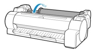
5. Hold roll holder by its flanges (A) and remove from roll holder slot.
