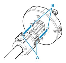
**3.** With leading edge of roll paper facing forward as shown, insert Roll Holder from right side of roll. Insert firmly until roll paper touches flange (A) of roll holder.
