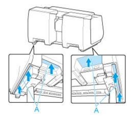
**2.** Remove tape and packaging material attached to the printer. Also open the top cover and remove stoppers and spacers inside the printer.
