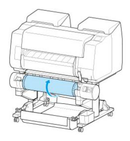
**6.** Change **Roll Holder Lock** switch on roll unit to release position.
