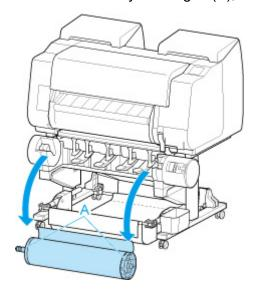
**10.** Push holder stopper lever (A) toward shaft to release lock, and while holding in position (B), remove holder stopper from roll holder.
