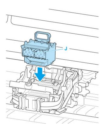
**16.** Grasp tab (F) of print head locking cover and lower it to front to lock print head.
