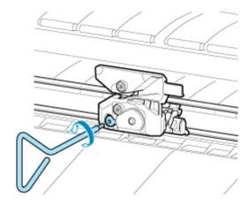
7. Remove cutter blade while holding D.
