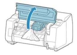
**3.** If the Carriage is out, move the Carriage to the left or right side, away from the jammed paper.
