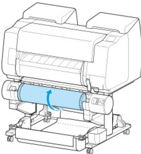
Apply adhesive tape to the rewound paper to hold it in place, if necessary.
