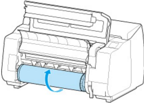
7. Hold Roll Holder by its flanges (A) and remove from roll holder slot.
