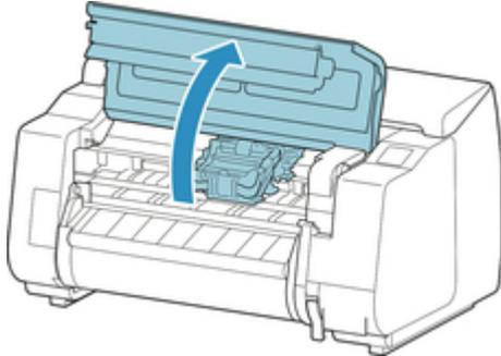
7. If the print head locking cover and print head lock lever are dirty, use a damp cloth that you have wrung out completely to wipe them clean.
