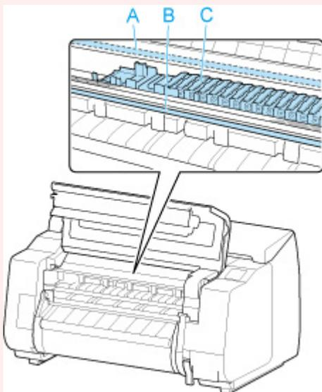
3. Place cut sheet with the print side up, insert in portrait orientation between platen (A) and paper retainer (B), and align paper's far edge using the following steps.
