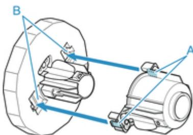
4. Insert paper core, which is for winding roll paper, into roll holder.
