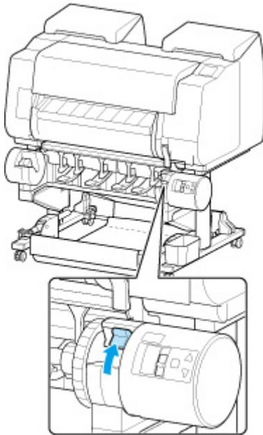
3. Hold flanges (A) so that roll holder's black gear is on left, align roll holder shaft with roll holder slot left and right guide grooves (B), and load.
