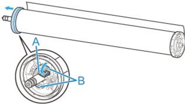
11. Remove printed material that has been taken up, from roll holder for each paper core.
