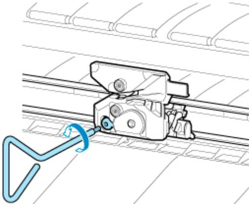
7. Remove cutter blade while holding D.
